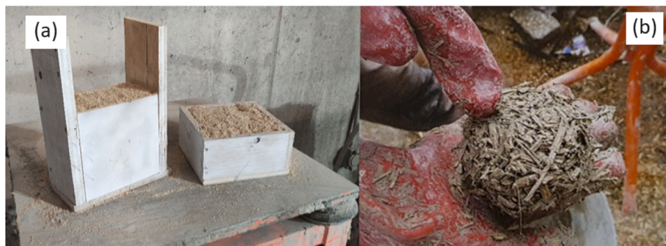
Fig. 2. The molds filled with HLC were placed on the vibration table (a) to produce the samples and the test ball method (b) [29].
