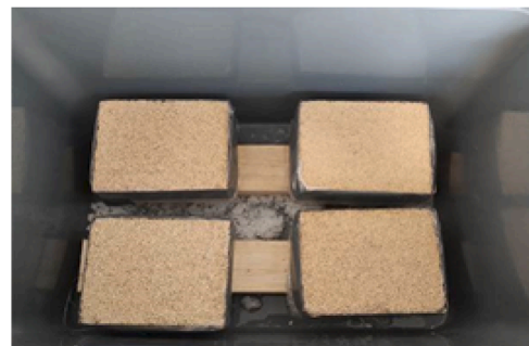
Fig. 5. Test assembly and setup of hemp-lime samples in a climate chamber for MBV testing.
